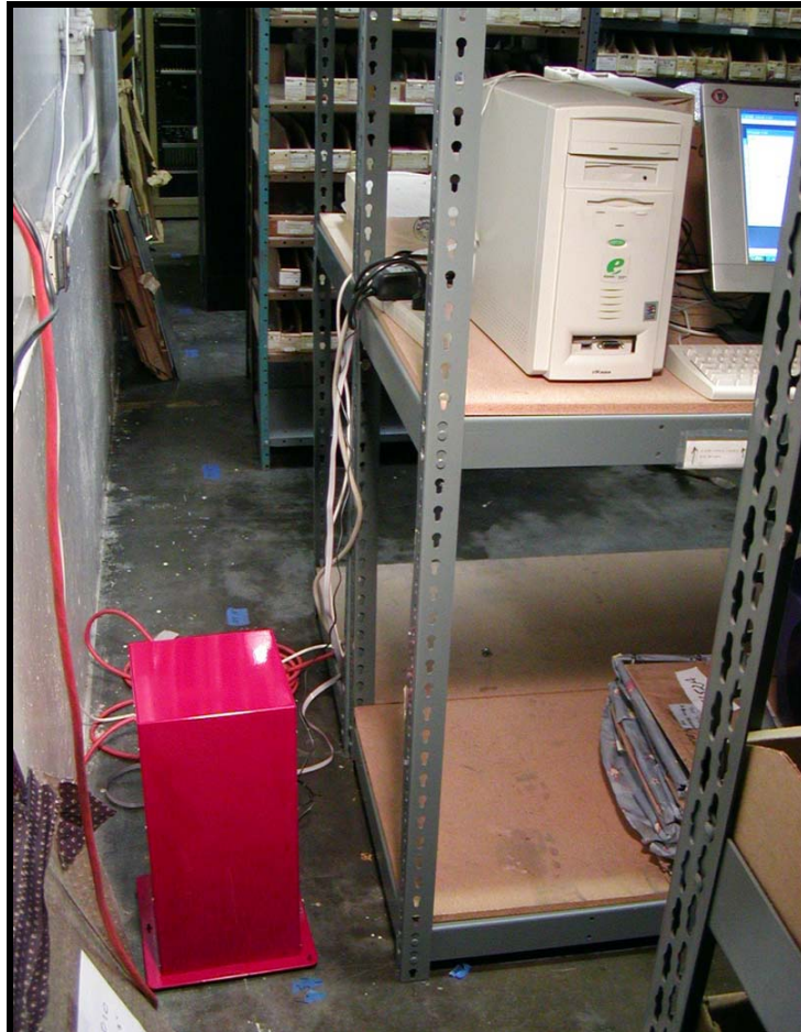
VolksMeter test site: On concrete slab in low-traffic area of RLL Instruments / Zoltech Corporation warehouse
